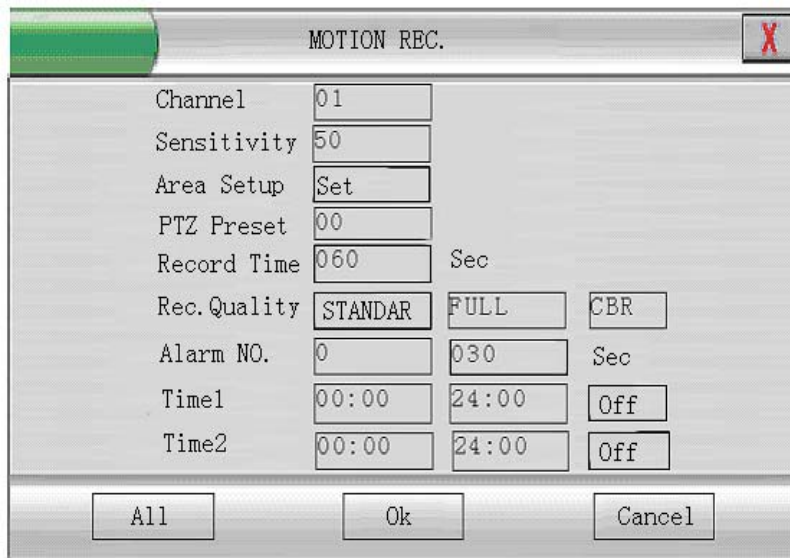
Figure 33 Motion Detect Record Setup
