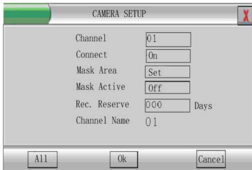
Figure 39 Video Channel Connections Setup
